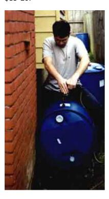
Step 1: Drill three of four holes in the barrel. One of these is for the bibet to connect your garden house to the barrel and the other fittings will allow you to add more barrels in the future. One of the barrels must have an overflow fitting near the top of the barrel. If you plan on using 3/4 inch fittings use a 1 inch hole saw to cut the holes. If you have an adjustable hole saw make it a little smaller than 1 inch.
