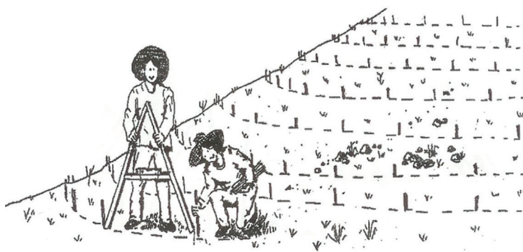
Figure 2: Laying out a contour line.
