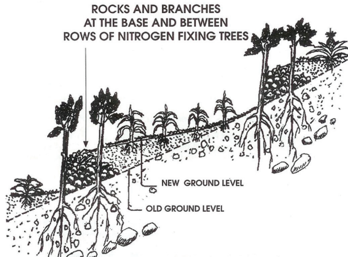
Figure 8: Build-up of terraces over time with the SALT system.
