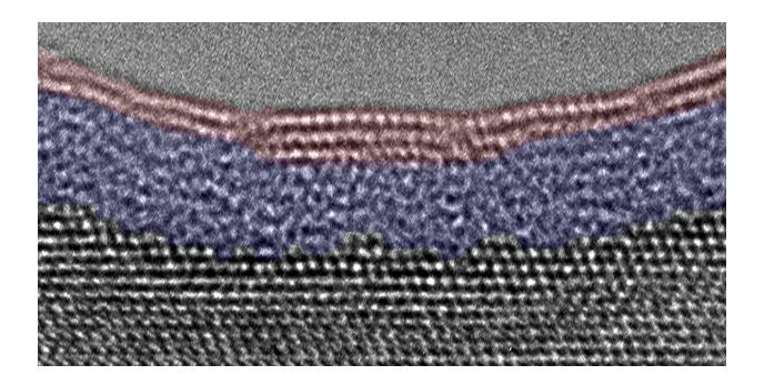
A transmission electron microscopy image of the oxidized aluminum surface shows that the passivating oxide film formed in water vapor consists of an inner amorphous aluminum oxide layer and an outer crystalline aluminum hydroxide layer. Credit: Provided.
